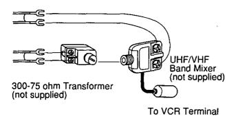
If your TV has both post and plug-type VHF terminals, the post connection is recommended to minimize signal loss.
