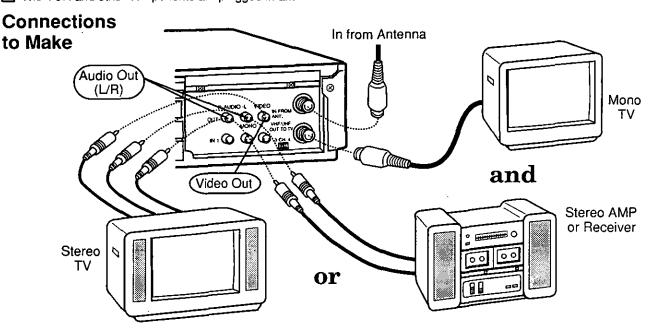
When recording, you may monitor in stereo, by connecting the VCR to either a stereo TV, or a mono sound TV with an external stereo amp and speakers.
