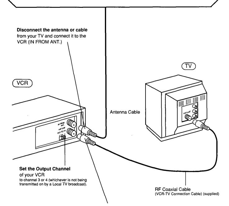
Connect the VCR to your TV with the RF Coaxial Cable (OUT TO TV).
